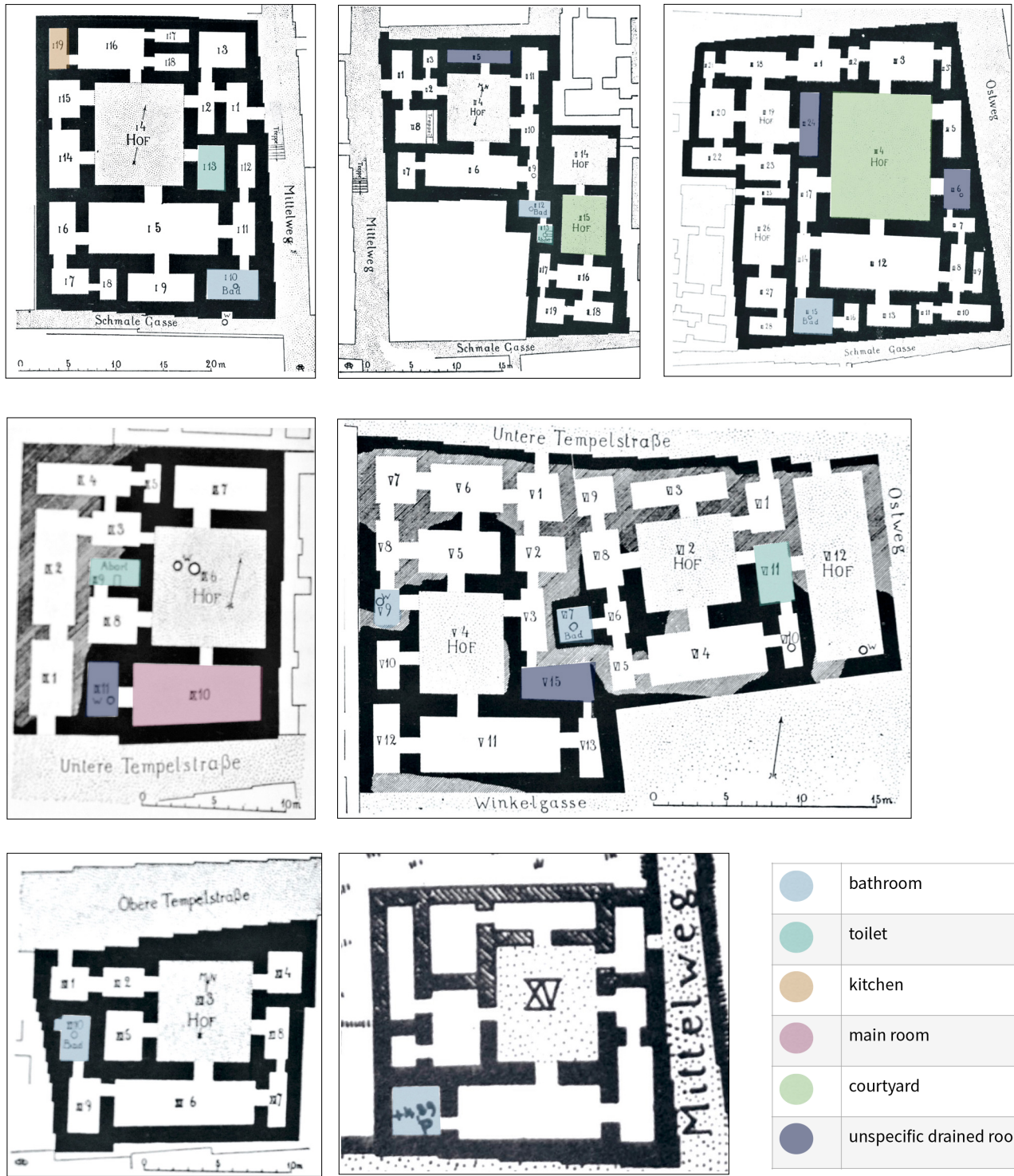
Figure 1 Overview of the rooms with drainage facilities in the 18 investigated dwellings in Babylon, based on Reuther's excavation report (Reuther 1926a)
