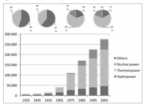
Figure 1. Transition in output from each power resource in Japan (FY)
