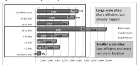
Figure 6. Development of hydropower generation in Japan
