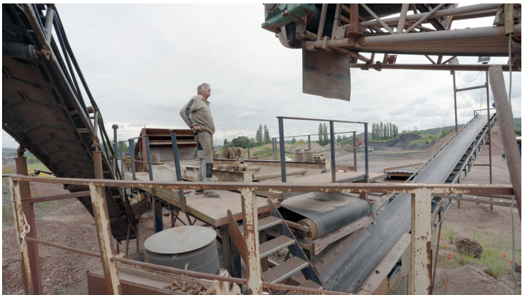
Figure 5 View on the conveyor belts used for processing shale
